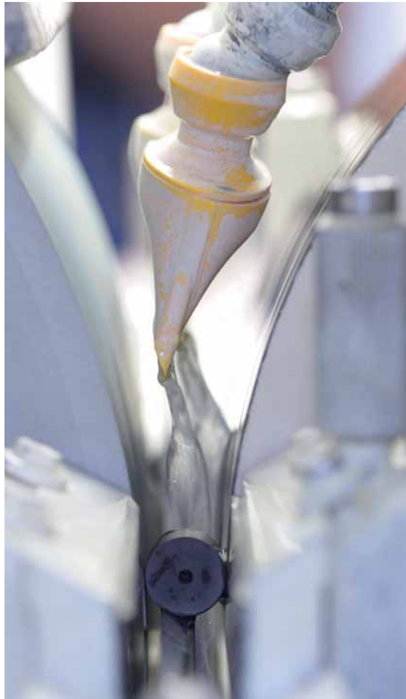
Centerless, cylindrical grinding of piezoceramic rods
