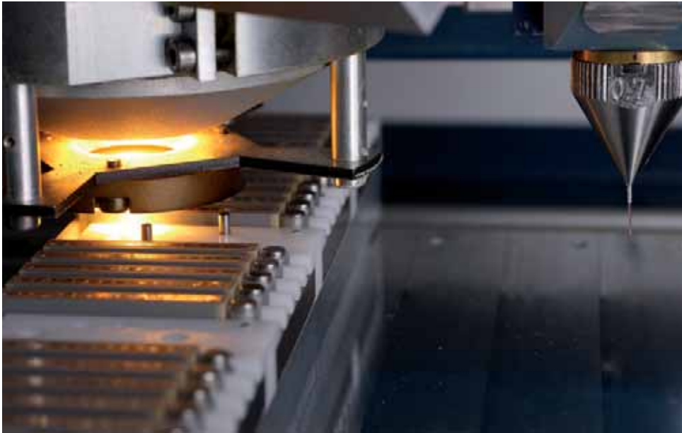
Automatic soldering machine with PICMA® actuators
